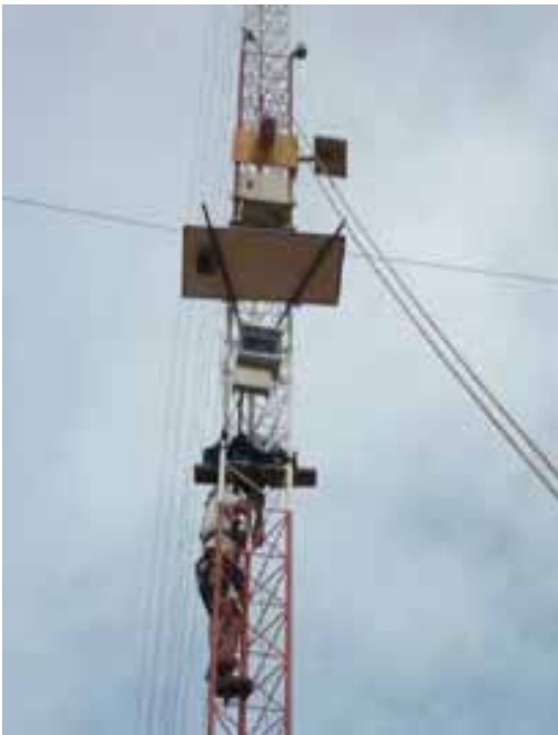
Figure 26: Equipment installed on a wind test tower in the Tera Kòrá wind farm and used for registration of sounds emitted by bats ('active monitoring')
